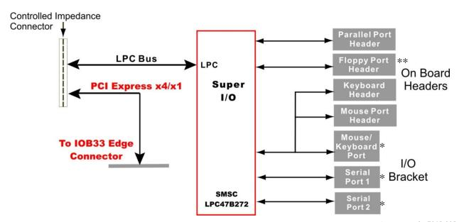
\*Except on the 7015-005 versions of the IOB33 \*\* The floppy port header on the IOB33 is not functional when using the IOB33 with the THD8141 SBC.
