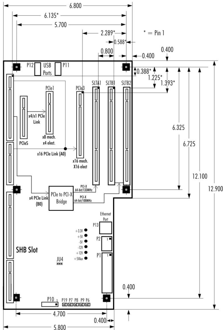
\*IOB31 required to provide PCI Express link to PCIe1 slot
