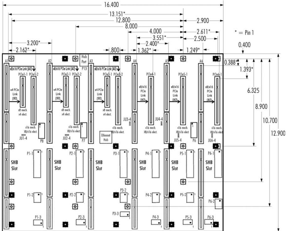
**Note:** Connectors and components on the layout drawings shown in dotted lines may or may not be populated on your specific model of the BP6FS66005 backplane. Refer to Backplane Configuration Table.
