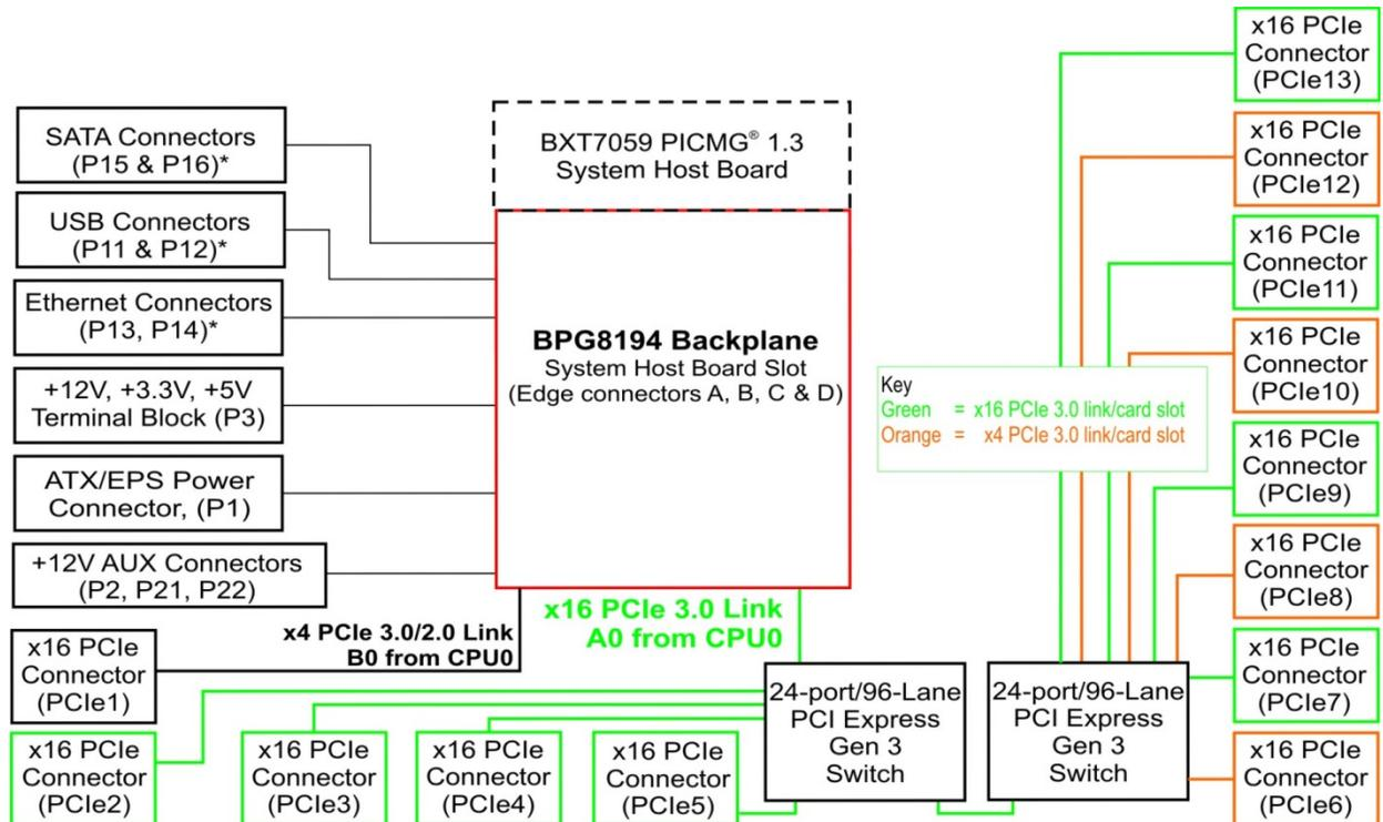
The SHB slot on the BPG8194 backplane supports any standard PICMG<sup>®</sup> 1.3 system host board. The backplane's PCI Express<sup>®</sup> interfaces were designed and manufactured using proper link routing techniques optimized for PCI Express Gen3 interfaces. The BPG8194 link design ensures maximum link speeds and data throughput between the system host board and standard PCIe plug-in cards regardless of the backplane slot distance from the system host board.
